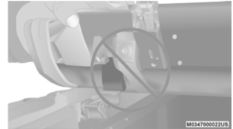
Incorrectly Seated Retainer
