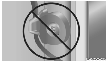
Incorrectly Seated Tailgate Strap
